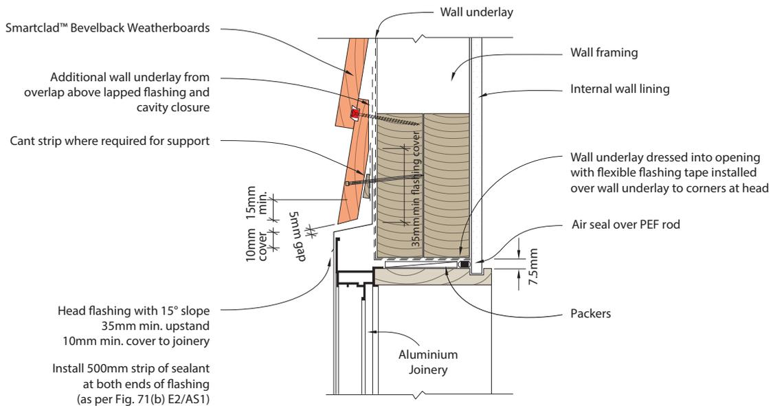
In very high and extra high wind zones, sealant must be installed between underside of head flashing and top edge of window head flange. — see E2/AS1 Fig. 71(c)
