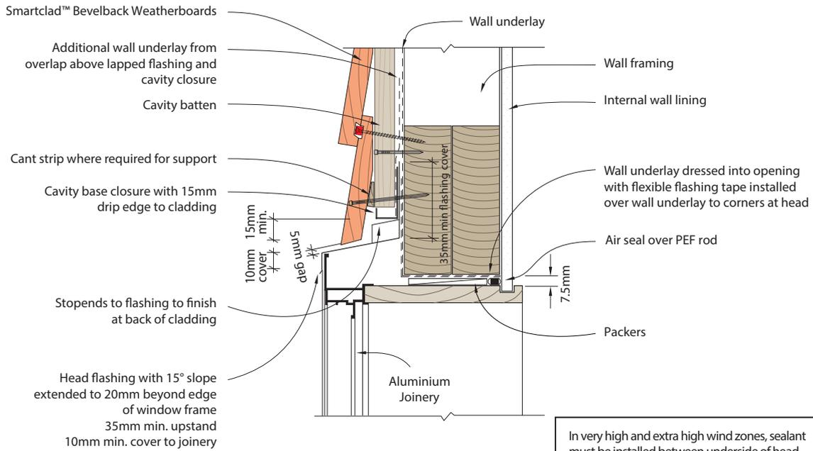
In very high and extra high wind zones, sealant must be installed between underside of head flashing and top edge of window head flange. — see E2/AS1 Fig. 71(c)
